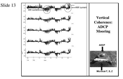
Acoustic Doppler Current Profiler (ADCP) data. Note x-axis is time and y-axis is current speed in centimeters per second. As you move from top to bottom of figure, water depth of each ADCP unit increases from the surface to 6 meters. This differs from the HF Radar image which only gives surface currents. The direction of the current is indicated by the direction the vectors are pointing.
