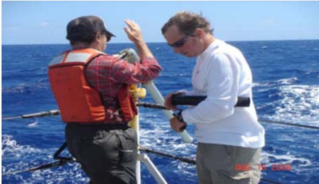
Photo 5: Sea Scholar, Sam Aceil , with instructor, A.J. Pearson , launching the XBT probe from the fantail area of the USNS Pathfinder .
