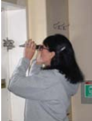
Photo 3: Carol Ann Drane is testing salinity using a refractometer.
