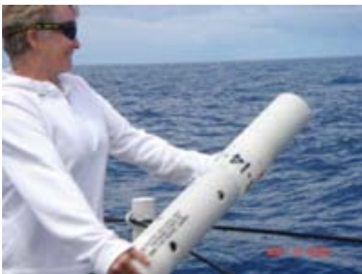
Photo 7: Saralee Lamb deploys the sonobuoy for acoustic testing.
