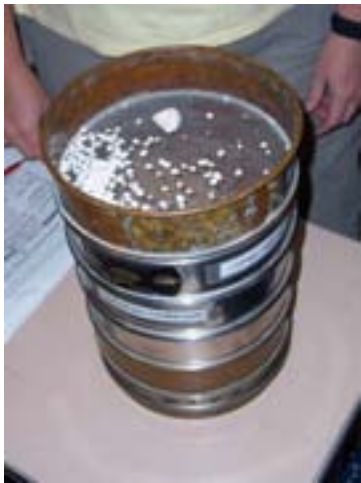
Photo 2: These are the graduated sieves used for sorting sand grain-size.
