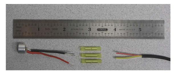
Hydrophone Cable Preparation: Complete steps 1 through 3 below for initial hydrophone cable preparations...
