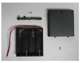
Phillips head screw, there are three plastic melted grommets securing the wire cover to the battery holder base. In prying off the cover, the heads of these grommets will snap off releasing the cover for removal. Set the wire cover and screw aside for later use.
