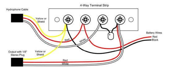
Note: if the hydrophone and output cables contain un-insulated shield wires, it is recommended to make them as short as possible to connect to the terminal while ensuring that no wire strands make contact with any other terminals.
