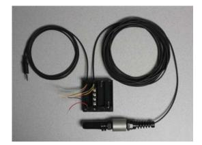
1) Working with both the hydrophone and output cables, strip back and remove approximately 3" of the outer cable jackets, exposing the
